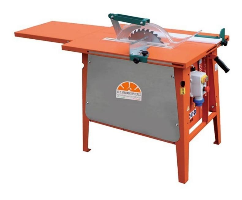
MANGUSTA bench saws are devised and designed to cut wood, chipboard, ply and building site planks and are excellent for all carpentry work and hobbyists. Motor with direct or belt transmission. The blade is equipped with a sheet metal protection hood. There is a magneto-thermal switch with release coil and immediate arrest button.
